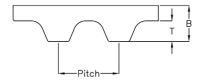
Height B mm= 2.7Height T mm= 1.2Length= 600Number of teeth= 120Pitch= 5Type= PU 50 AT5 600Width= 50
